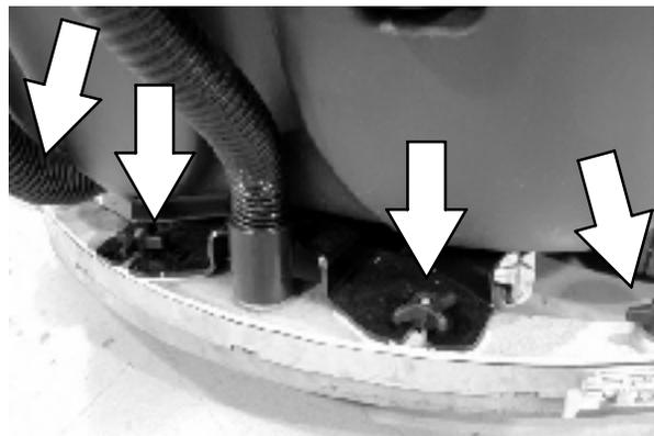
14. Reinstall the squeegee suction hose onto the rear squeegee assembly.
