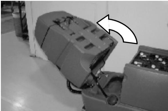
12. Flush the solution tank and rinse the float sensor located inside the back part of the solution tank. Rinse the screen filter on the bottom of the tank.
