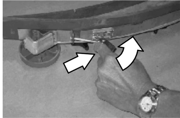
13. Reinstall the rear squeegee under the squeegee mount bracket and tighten all four knobs.
