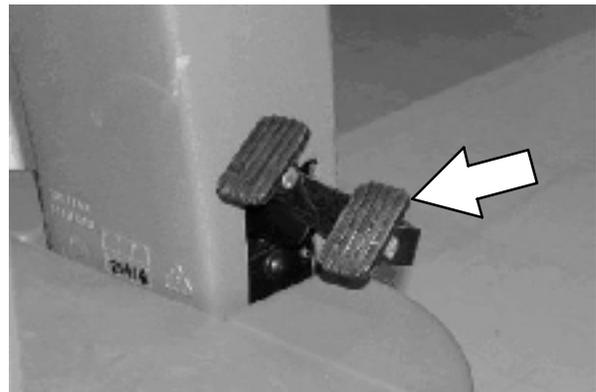
5. Release the *propel pedal* to stop the machine. Scrubbing functions stop and the automatic *park brake* will engage when the machine stops.
