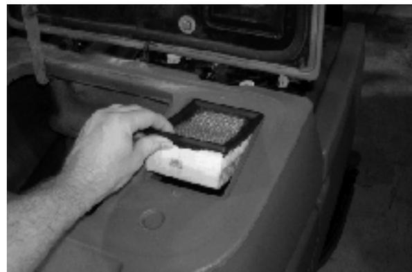
5. Lift the recovery tank cover. Flush the inside of the recovery tank with clean water.
