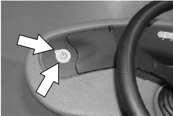
*NOTE: Open the control panel cover to adjust the Brush Pressure and Solution Flow Setting while scrubbing if necessary.*
