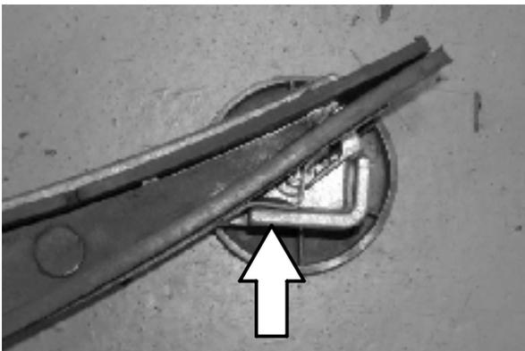
12. Tighten the rear squeegee retaining band tension latch.
