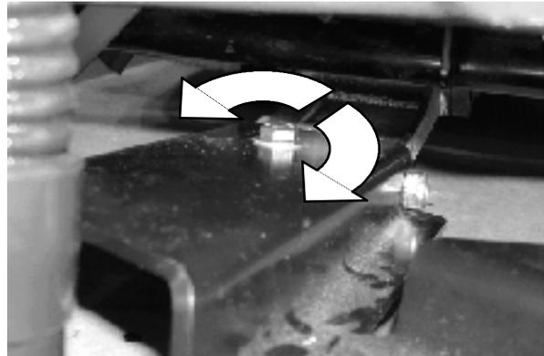
Turn the squeegee leveling bolt counter-clockwise to increase the deflection at the ends of the squeegee.
