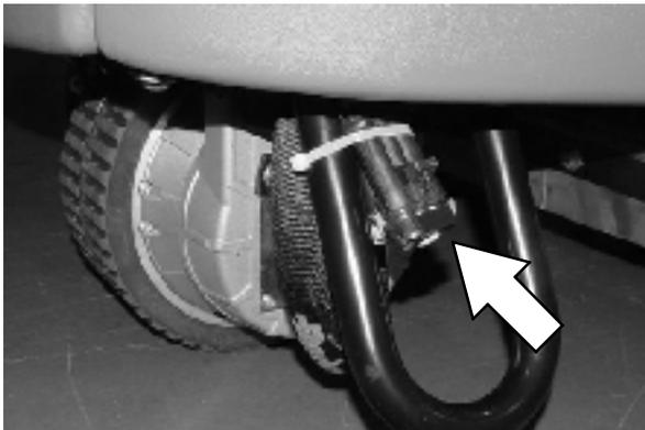
To disengage the brake, insert the tip of a small screw driver between the electronic brake lever and the hub.
