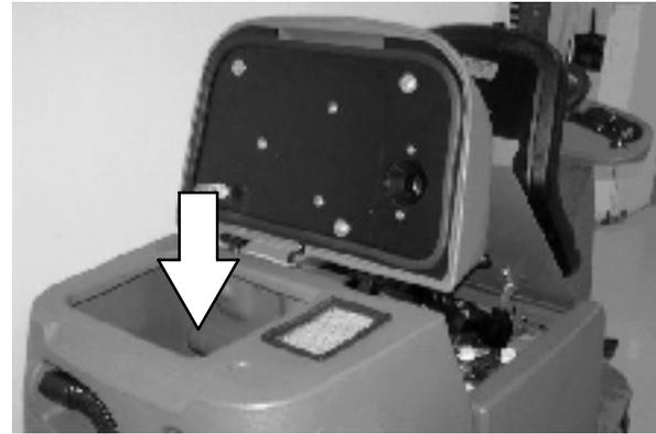
6. Rinse the float sensor located inside the recovery tank.
