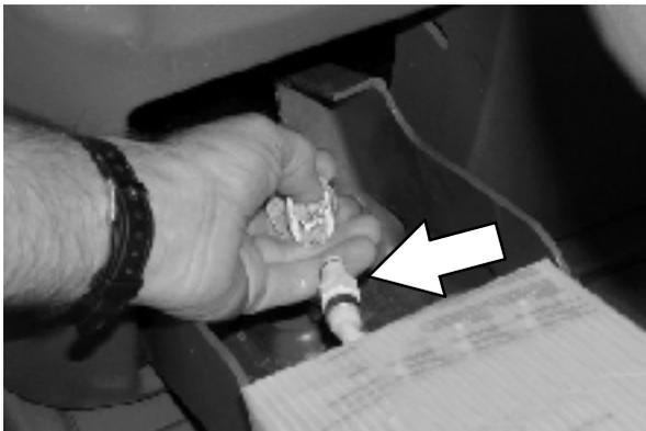
5. Remove the perforated knock outs from the new FaST-PAK carton. Do Not remove the bag from the carton. Pull out the hose connector located on the bottom of the bag and remove the hose cap from the connector.
