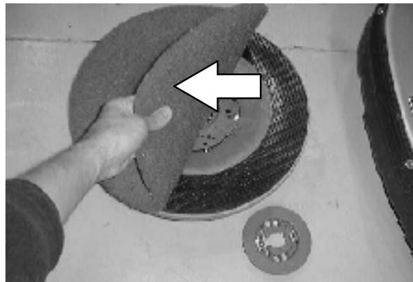
4. Reinsert the pad driver into the machine.
