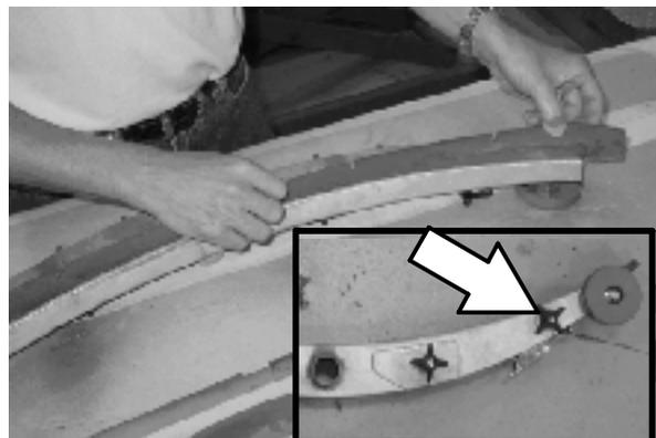
8. Install the new front squeegee blade or rotate the existing blade to the new edge. Be sure the holes in the front squeegee blade are hooked onto the tabs on the front blade clamp.
