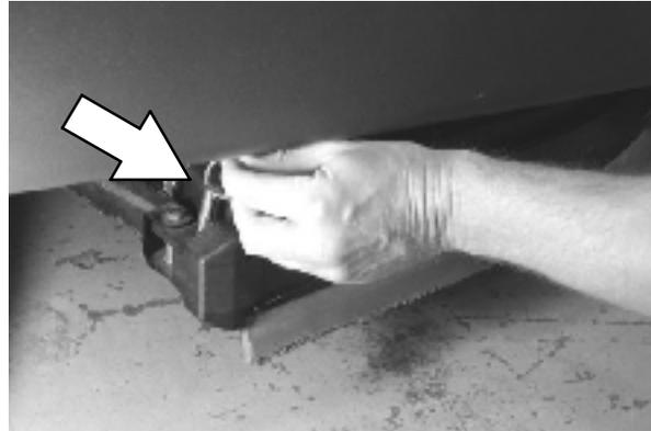
4. Open the side squeegee retainer pivot toward the front of the machine, then pull the side squeegee toward the rear of the machine to access the scrub brushes or pads.
