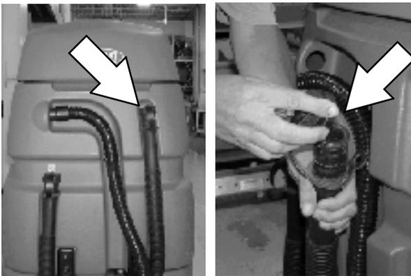
7. Replace the recovery tank drain hose cap and mount the drain hose back onto the mounting clip after the tank is drained.
