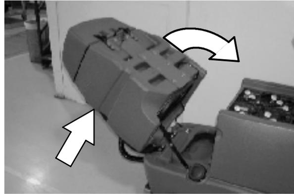
14. Unhook the seat latch and lower the operator seat.
