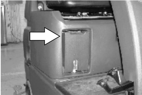
4. Squeeze the button on the FaST supply hose connector, then pull the empty FaST-PAK out from the compartment.
