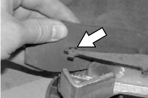
9. Lightly tighten the two outer knobs.
