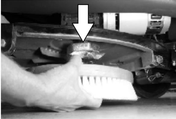
6. Place the new scrub brush/pad driver onto the drive hub. Ensure that it is securely mounted onto the brush drive hub.
