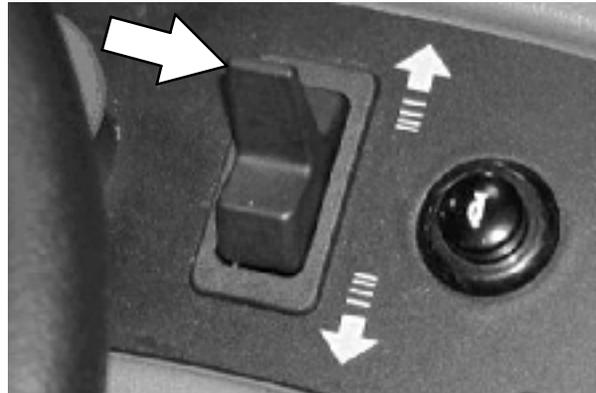
*NOTE: The squeegee automatically raises when the machine is driven backwards. This prevents damaging the squeegee. When the machine is placed in reverse, the vacuum fan will shut off after a short delay.*
