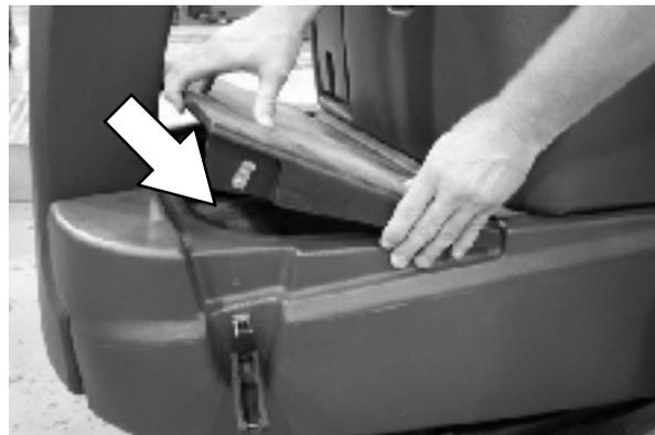
16. Replace the solution tank drain hose cap and mount the drain hose back onto the mounting clip after the tank is drained.
