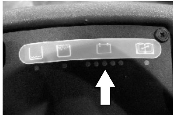
When the batteries are fully charged, all five lights are lit. As the batteries discharge, the lights go out until only the left light is blinking.
