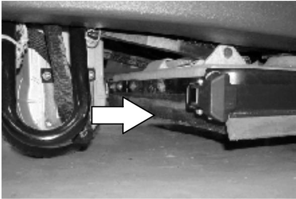
The skirts should clear the floor by 0 to 6 mm (0 to .25 in) when the scrub brushes are new and the scrub head is down.
