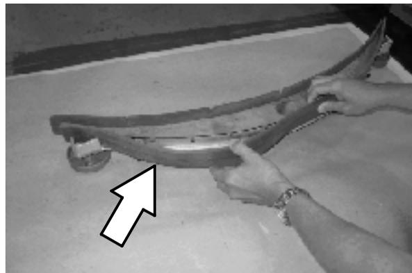
7. Loosen the two outer knobs on the rear squeegee assembly. Remove the front squeegee blade from the squeegee assembly.
