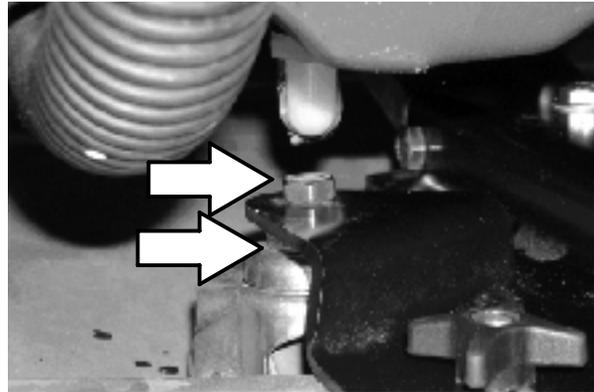
5. Drive the machine forward again to recheck the squeegee blade deflection after adjustments are made.
