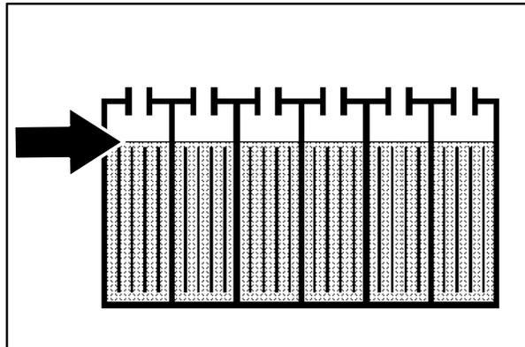
Using a hydrometer, measure the specific gravity to determine the charge level and condition of the batteries. If one or more of the battery cells test lower than the other battery cells (0.050 or more), the cell is damaged, shorted, or is near failure. Completely recharge the batteries and then retest.
