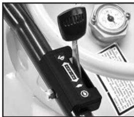
The operator throttle is conveniently located on the handle.
