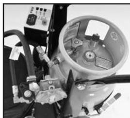
80% safety fill type propane tank. All propane system components are UL approved.
