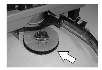
12. Line up the brush /pad driver socket with the drive plug.
