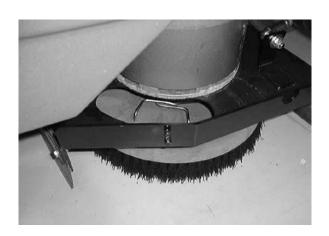
6. Press the brush/driver spring clip together with your thumb and index finger. The scrub brush/pad driver will drop off the drive hub. Pull the brush/driver out from under the scrub head.
