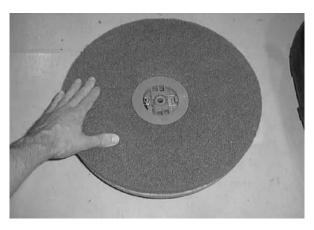
11. Place the new scrub brush/pad driver on the floor to the side of the scrub head. Push the brush under the scrub head.
