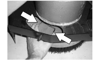
14. Check to make sure the brush is securely mounted on the brush drive hub.
